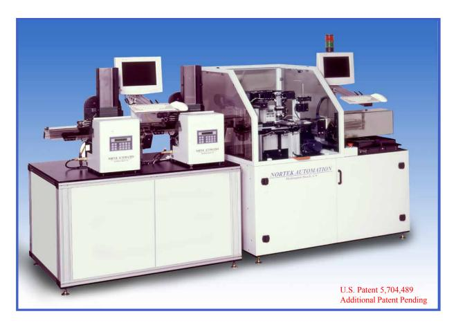
**GFH 2000C Test Handlers**Magazine-fed boards are tested and then placed on conveyor
