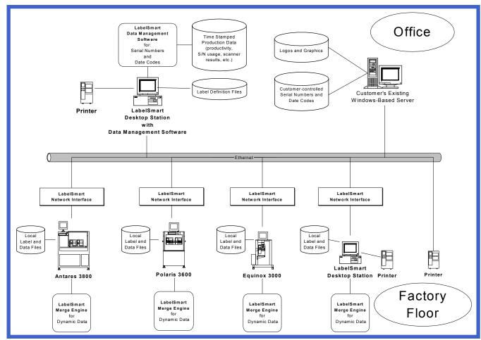
Nortek's LabelSmart Software Suite is a modular label creation system designed for Nortek's line of label applicators. The package provides a consistant look-and-feel to each station. Label data, including serial numbers and date codes, can be maintained locally or over a network. LabelSmart can be used on a single machine or as a plant-wide standard.
