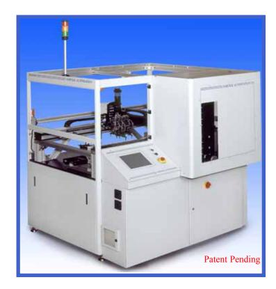
Nortek's revolutionary multi-site Memory Module test handler was designed to minimize handling prior to test. Individual modules enter the system via conveyor or tray. They are scanned, picked-up and inserted into test sites. Modules are then sorted into pass or fail trays. Up to ten empty pass trays can be held in queue while the system is in operation. An Automatic Labeling and an Automatic Depaneler System can be added to further reduce manual handling.
