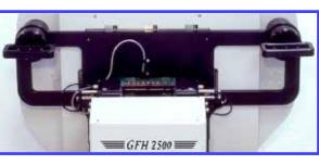
The GFH 2500 high Speed Test Handler was designed for high speed testing of SIMM/DIMM/RIMM/SODIMM Memory Modules. First gravity fed handler to employ a high speed connector utilizing industry standard sockets for testing SDRAM modules at 133+ MHz speed.
